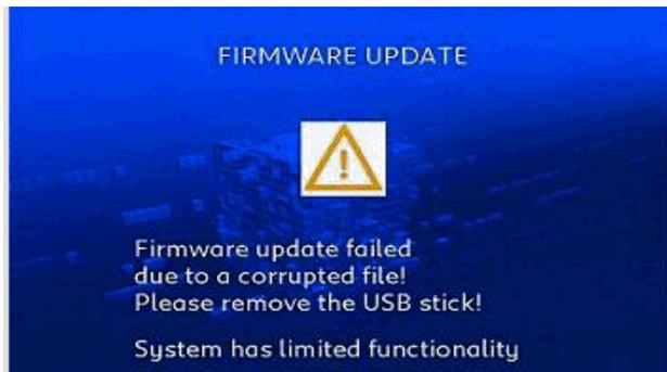
If the update is not fully completed, the following message appears: "FIRMWARE UPDATE FAILED DUE TO A CORRUPTED FILE".
